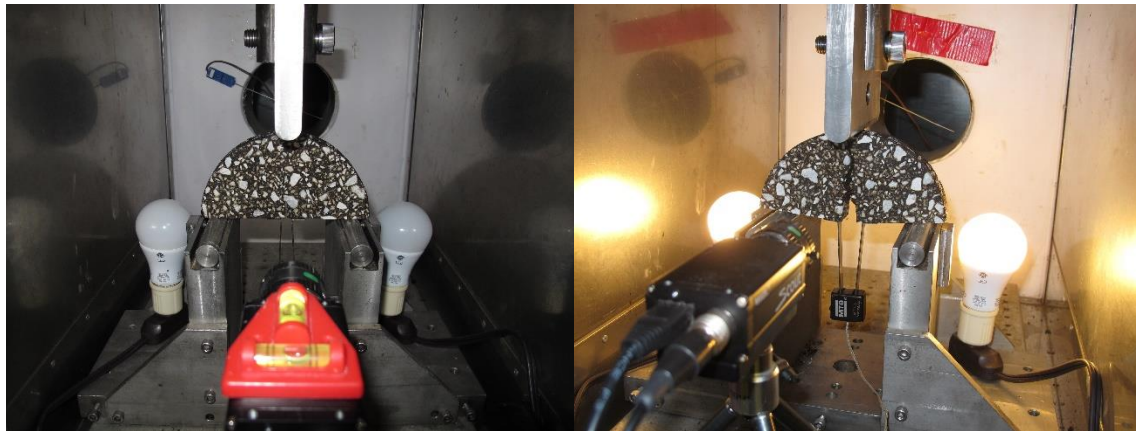
Figure 4.3 SC(B) Test Configuration, Before(left) and After(right) Test
